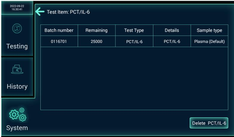
d) Item deletion: Select the item parameter which is expected to be deleted according to the actual need.
