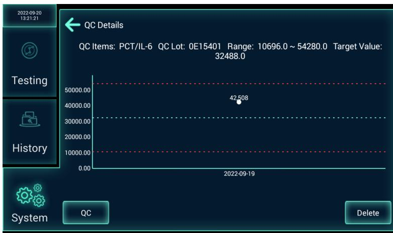
QC results should be within the given target range. Quality control frequency: It is recommended that users perform reagent quality control at least once per batch.
