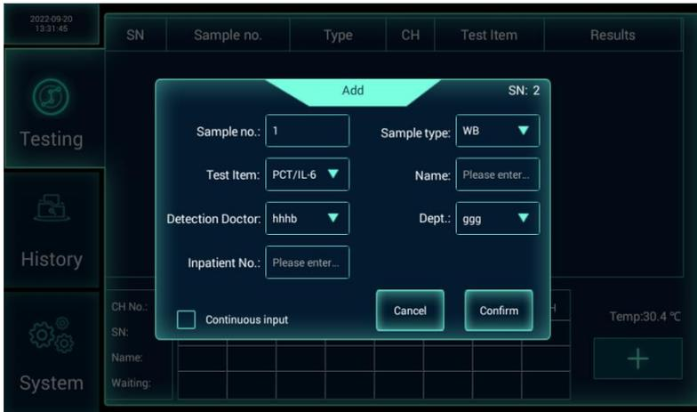
Dilute the sample and add it to the test cassette according to the instructions of the reagent, insert the cassette into the free channel of the 8 channels.
