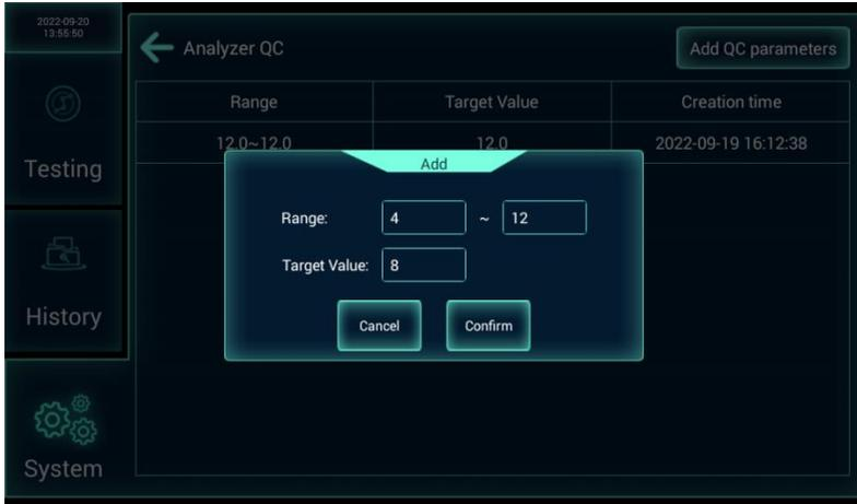
After entering the QC parameters of the quality control card, click “Confirm” to add the quality control parameters.
