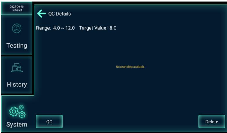
Click "QC" to start the analyzer quality control. QC results should be within the given target range. Quality control frequency: It is recommended that users perform analyzer quality control at least once a month.
