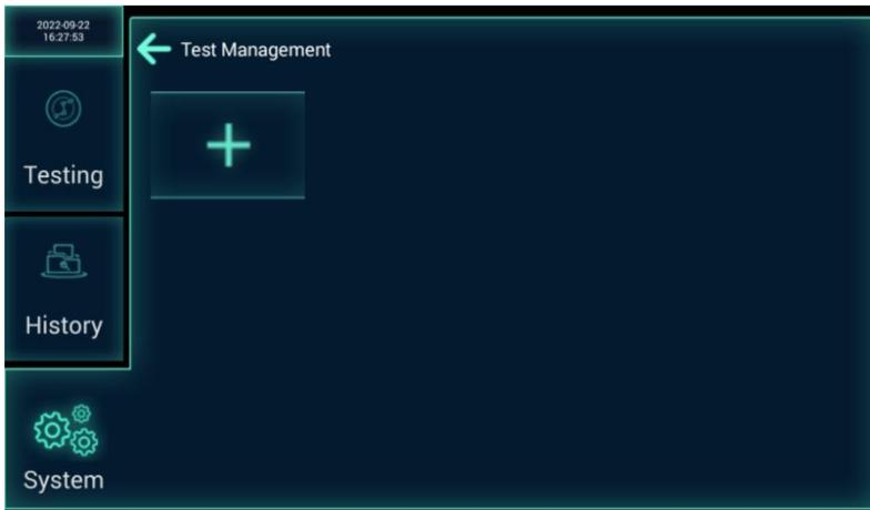
Insert the reagent information carrier that comes with a supporting kit, click the “+”, the analyzer will read the information in the carrier
